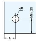
Boring position changes with the glass thickness.
